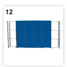
11-12. Unroll the graphic panel to its full lenght and attach it to the metal bars. The edge of each panel will be positioned on the middle of the metal bar, the other half remaining free for attaching the next panel.
